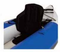
For the rearward seat, clip the back straps to the spray skirt D-rings and the foward straps to the D-rings just in front of the seat. For solo paddling, position at the midpoint of the kayak.
