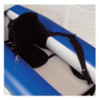
Clip the strap to the floor strap D-ring nearest your feet and clip the other end to the seat D-ring. One strap goes on each side of the kayak. They have an elastic helper that takes up slack when you are not pulling against the strap.
