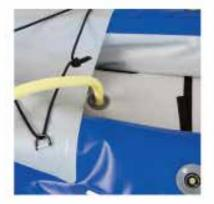
Partially inflate the sides and the floor and check that the floor is tucked underneath the sides. Finish inflating the floor then sides. Working pressure of the sides and floor is 3.2 psi. The floor can be inflated up to 14 psi but is not necessary to do so.
