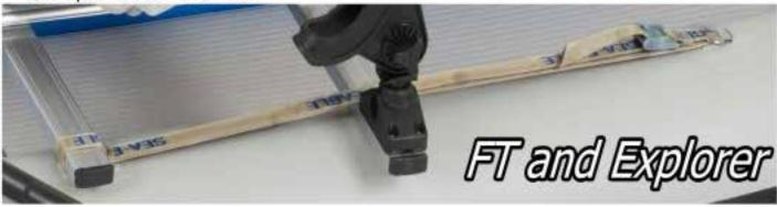
**Tandem** 465FT shown here with optional motor and motor mount. The strap goes under then over the front bar and over the rear rod holder bar. The front D-ring is just behind the bar.
