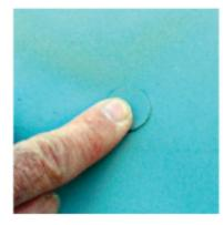
Mate the patch to the boat and smooth down until the patch adheres. Do not inflate, allow at least 24 hours to cure before inflating.
