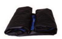
Keep folding until nearly up to the valves, then begin folding from the bow. Fold the halves together and place boat on its bag. The straps will help compact the boat.
