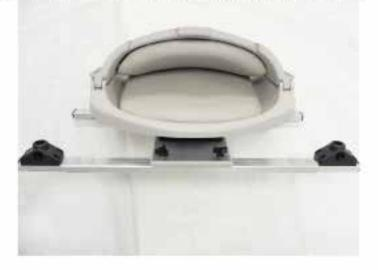
Set the frame on the boat with the front bar just in front of the middle D-rings.
